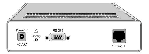
Figure 2-5: LanProbe's Rear Panel
